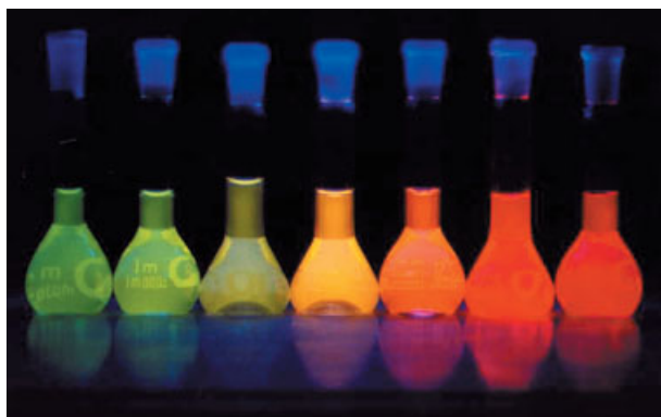
Fig. 2.3 Size-dependent luminescence of colloidal semiconductor nanoparticles. The emission color of thiol-capped CdTe nanocrystals can be adjusted by their size (2.5–4.5 nm range) to be green, yellow, orange or red; the room temperature quantum yields of the luminescence are up to 40% [6].
