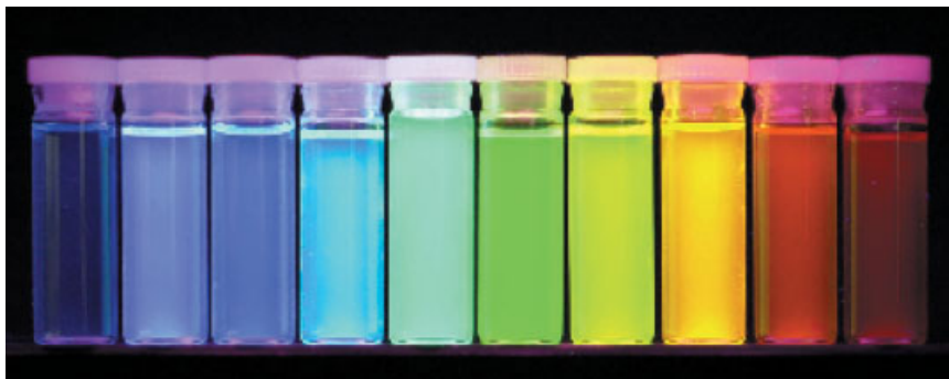
Fig. 16.1 Ten distinguishable emission colors of ZnS-capped CdSe quantum dots excited with a near-UV lamp. From left to right (blue to red), the emission maxima are located at 443, 473, 481, 500, 518, 543, 565, 587, 610, and 655 nm (adapted with permission from Han, Gao, Su, and Nie, Nat. Biotechnol. 19, 631, 2001).
