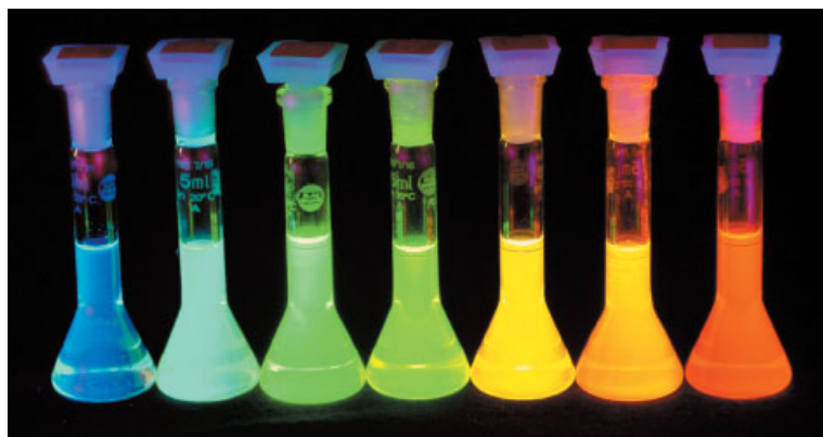
Fig. 2.18 Size-dependent change of the emission color of colloidal solutions of CdSe/ZnS core-shell nanoparticles. The particles with the smallest ( \sim 1.7 nm) CdSe core emit blue, the particles with the largest ( \sim 5 nm) core emit red.
