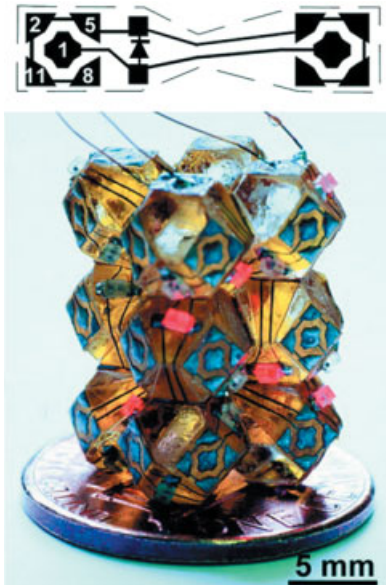
Fig. 14.5 Example of an electrical circuit assembled via capillary forces from prefabricated components. The building blocks are millimeter-sized polyhedrons made from flexible plastic. The pattern of contact pads on the surface and the connection diagram for the internal LED are shown on top (excerpted from [53] with permission; copyright American Association for the Advancement of Science, 2000).
