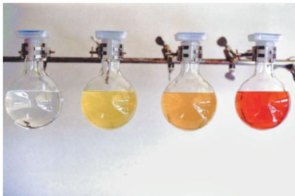
Fig. 2.2 Manifestation of the size-quantization effect as a color change of aqueous colloidal solutions of CdSe nanoparticles. The particle size changes from left to right from \sim 1.5 to \sim 4.5 nm.
